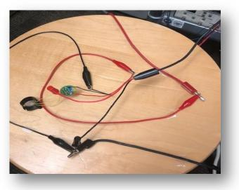
A feedback circuit setup used to find the resonance frequency by using the signal generator.
