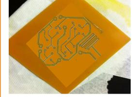
etching solution and agitate until all the copper has dissolved (30 min.). Step 9: Rinse in water bath. Let It dry and rinse thoroughly with rubbing alcohol.
